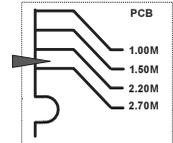
For reducing the detection range, slide the PCB up or tilt the swivel down.
