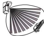
For optimum detection, select a location that is likely to intercept an intruder moving across the coverage pattern at a 45° trajectory.
